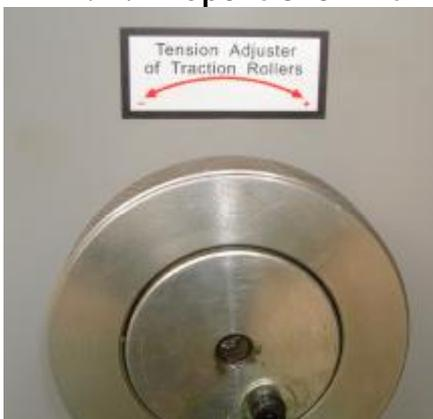
Tension adjuster of traction rollers:
